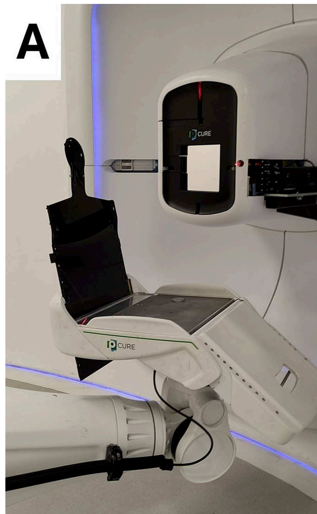
Fig. 1. The Patient Robotic Positioning and Imaging System (P-ARTIS): A. A leg-up chair for head and neck patients. B. Illustration of the P-ARTIS coordinate systems: the treatment Z-axis is always orthogonal to the floor, while the imaging Z-axis is parallel to the axis of the sub-vertical 4DCT slider.
